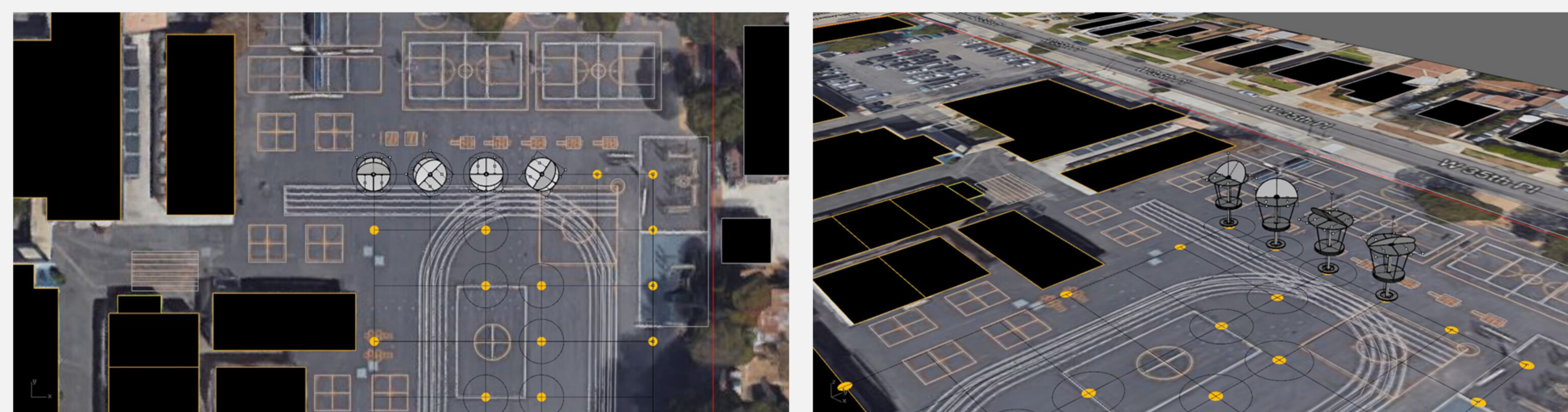
Top: 3D shade analysis of shade cover at Bright Elementary throughout the day with the addition of the proposed shade structures. These models were compared to shade analysis of the site prior to the addition of the shade structures, in order to demonstrate the impact of the structures on shade cover in the playground. There is a significant increase in shade cover when the structures are added. Bottom: Detailed 2D and 3D site models of proposed shade structures, with blacktop designs and building footprints for context.
